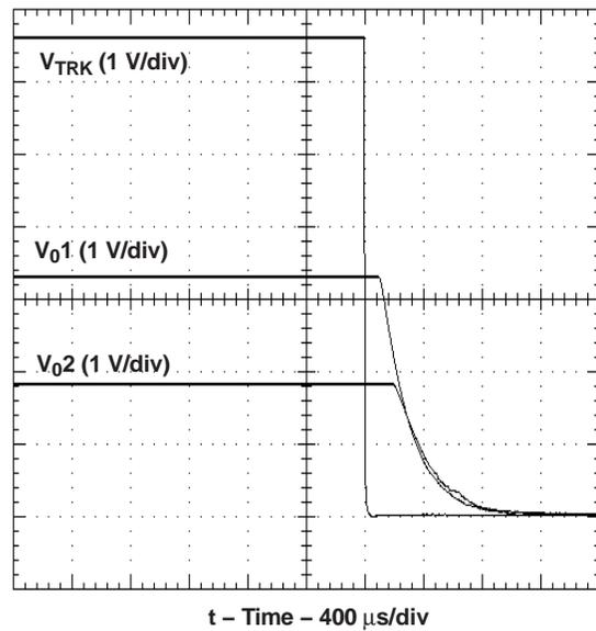
Figure 15. Simultaneous Power Down with Auto-Track Control
