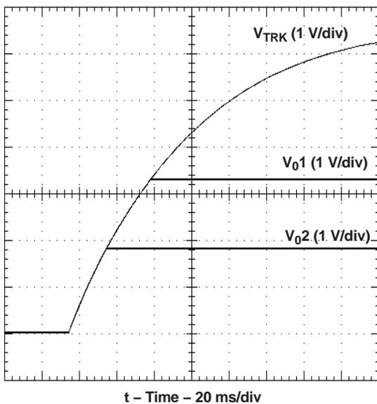
Figure 14. Simultaneous Power Up With Auto-Track Control
